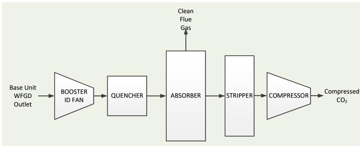
**Figure 2-1: CO<sub>2</sub> Capture Block Diagram**
